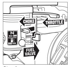
**Step 6** Slide the throttle control to the fast position. Move the choke lever to the "CHOKE" position (only if the engine is cool). After starting, move the choke to "RUN". Turn fuel valve on.
